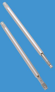
The 5278 internal thread restorers where developed to allow M12 and M14 sparkplug threads to be restored from the inside of the engine outwards without removing the cylinder head so ensuring that any debris and carbon deposits come out with the tool.
