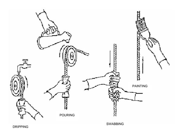
Figure 1. Methods of FLUID FILM LIQUID A application include dripping, pouring, swabbing and painting. When the rope is bent, the LIQ. A will penetrate much easier. Arrows indicate the direction of the rope's movement.
