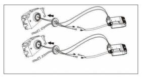
After installation of all cables and ballasts, check correct operation of the new light source in your car - xenon headlights. <u>Note:</u> If both lights do not turn on at the same time, replace the battery with a more powerful one with a capacity of 60Ah because the problem may be too small tension of ballasts. Replace fuses of headlights to have a value of at least 20A.
