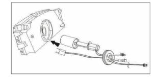
5. Reinstall the plastic cover after putting wires in drilled hole and seal connection with rubber ring installed on the cables.
