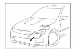
2. Remove the old halogen lamp located in the back of the reflector (after removing the plastic cover).
