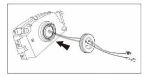
6. Install the connection following the picture below. Install ballasts in the nearest possible place next to the reflector using cable ties or attached coasters. Remember to locate highvoltage cables away from other electrical wirings. Otherwise, there may appear interference in electronic systems of the vehicle.
